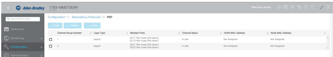
Figure 33 - Stratix 5800 PRP Configuration
